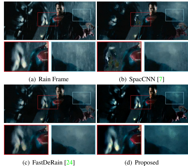
Figure 1. Visual results of different deraining methods. Compared with FastDeRain [24] and SpacCNN [7], our method is better at removing rain accumulation and accumulation flow (blue box) with less detail loss (red box).
